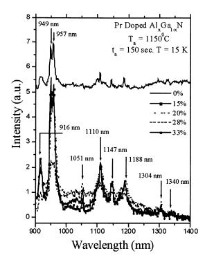
Fig. 4. PL spectra measured at 15 K for the Pr-implanted GaN epilayer and the  $Al_xGa_{1-x}N$  alloys. The spectra are vertically displaced for a clear presentation.
