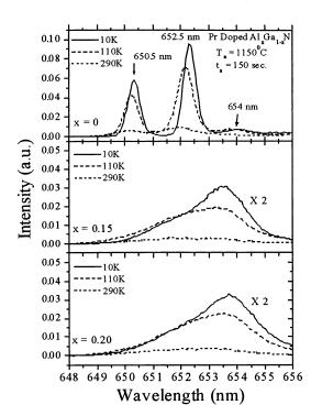
Fig. 2. PL Spectra measured at three representative temperatures 10, 110 and 290 K for the Pr-implanted GaN epilayer, the  $Al_{0.15}Ga_{0.85}N$  alloy, and the  $Al_{0.20}Ga_{0.80}N$  alloy.
