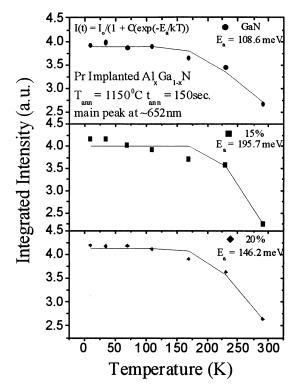
Fig. 3. PL integrated intensity vs. temperature in the 650 nm region by Eq. (1). The equation of fitting reveals the thermal activation energy for the Pr-implanted GaN epilayer and  $Al_xGa_{1-x}N$  alloys studied.
